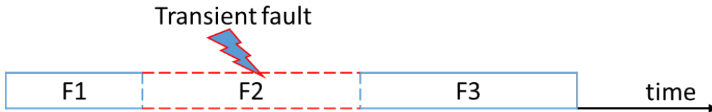
Figure 4.12: A transient fault appears and disappears on a PE component.
