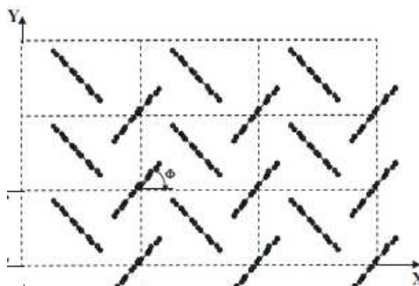
Figure 39 Herringbone crystal structure of PPV in the x and y directions, (taken from reference [50]) Where \Phi=52^\circ
