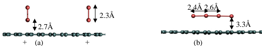
Figure 27 Optimised geometries of 2Br 2 on graphene (a), Br 4 on graphene (b) and above is the hypothetical reaction for the thermodynamic transformation.
