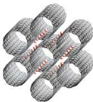
Figure 23 SWCNTs bundle showing specific interstitial spaces for Br intercalations (image taken from Ref. [40])
