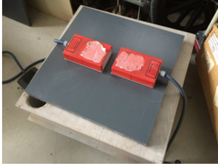
Figure 4.19: GPR experimental set-up conducted with the CMP-TE configuration of antennas on PVC+limestone slabs
