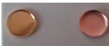
Figure III.2.4 – Joints DSC haute pression.
