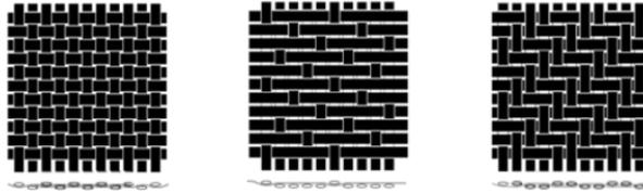
Figure I.2.4 – Exemple de tissus composites [3].
