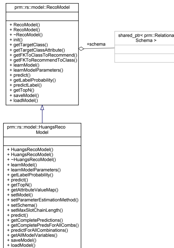
Figure 9.9 – Class diagram of RecoModel
