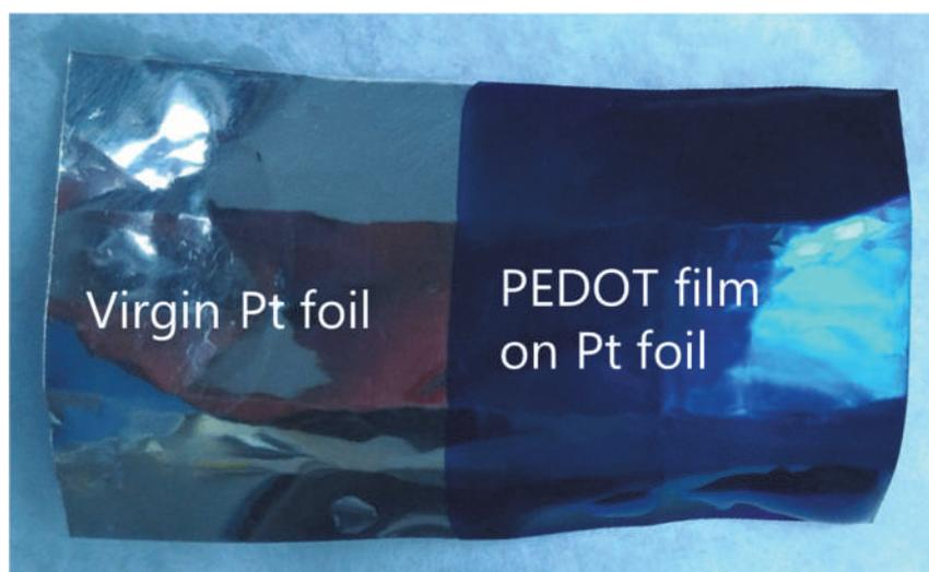
*Figure II.14. PEDOT film electropolymerized on a Pt foil during 500s at 0.80 V vs SCE.*
