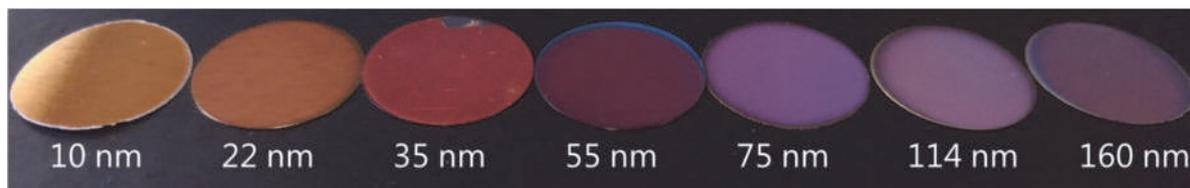
*Figure II.3. Au metallized AAO porous membranes of different pore diameters.*
