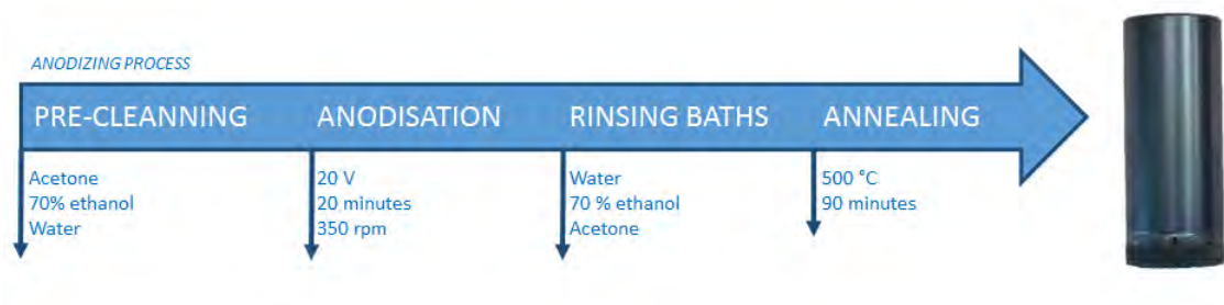
Figure 4.11: The different steps in the anodizing process with its parameters and its final blue-coloured appearance
