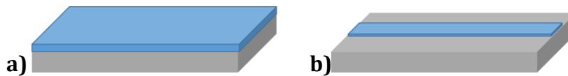
Figure 1.2: Two different kinds of waveguides. Planar waveguides guide light only in the vertical direction, whereas channel waveguides guide in two dimensions.
