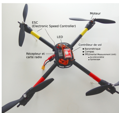
FIGURE 2.2 – Composants d'un drone.
