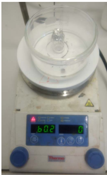
Figure 4.11: Solvent chamber setup for binder activation treatment
