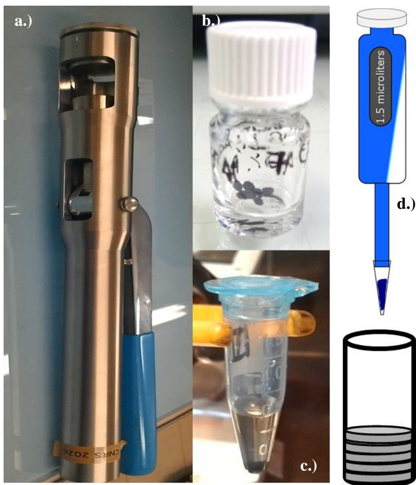
Figure 4.1: Pellet press (a), pellets (b), oversoaking scheme(c), and in rotor soaking scheme (d).
