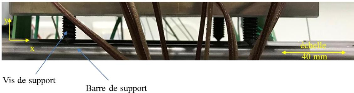
**Figure IV-6:** Supports de l'élément test.
