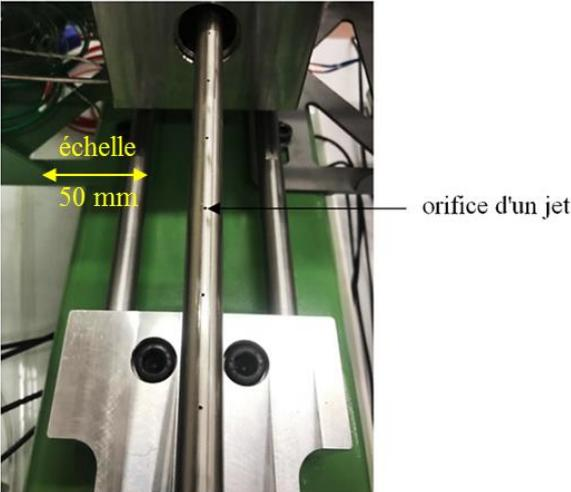
Figure IV-15: Orifices des jets.
