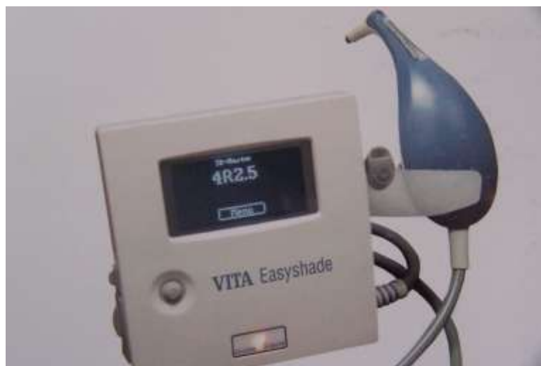
Figure n° 7: appareil VITA Easyshade (photographie Dr. Y. Amouriq)
