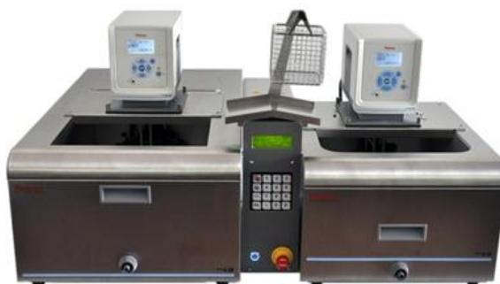
Figure 41 : machine de thermocyclage (Certiga-TCS-30)
