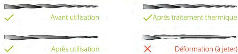
FIGURE 27 - LE TRAITEMENT THERMIQUE APPLIQUE POUR RECUPERER LA FORME ORIGINALE DE LA LIME EST DE TYPE CYCLE DE STERILISATION (157)
