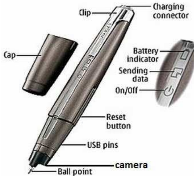
Figure 3-12: Features of a digital Pen, Nokia SU-1B
