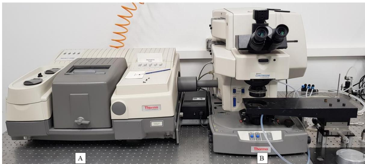
Fig.I.7: A) Nicolet FTIR 5700 spectrometer at LPG; B) IR microscope equipped with the X15 Cassegrain objective
