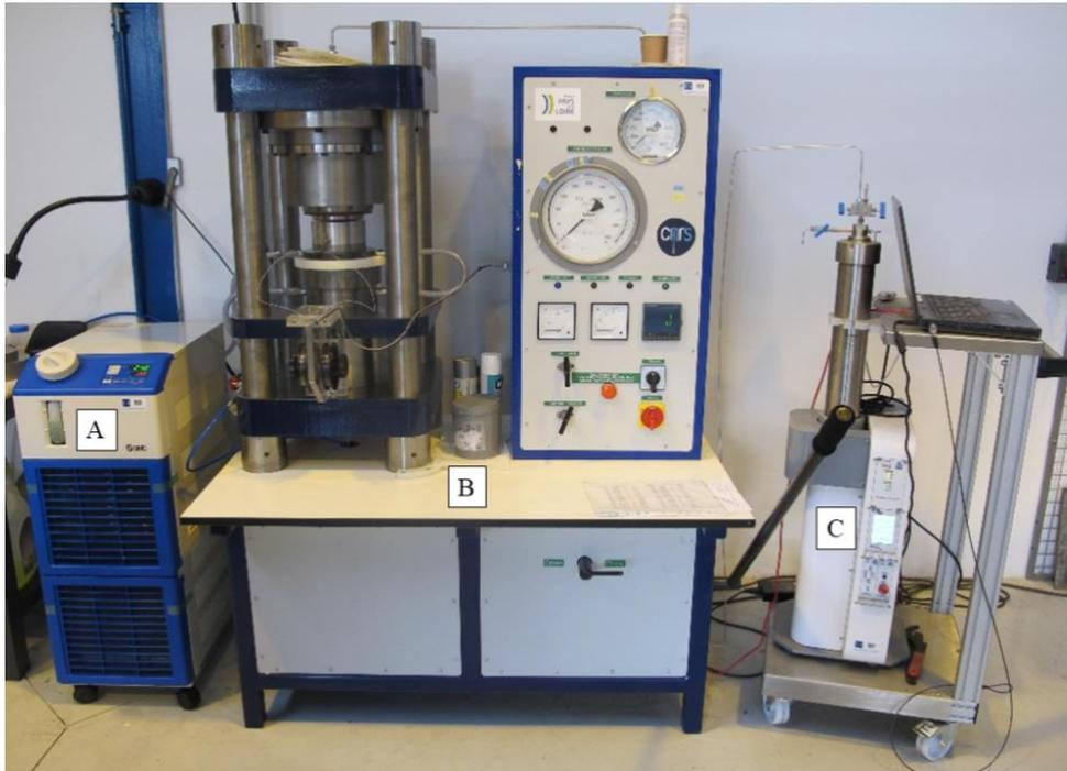
Fig.I.1: A) Chiller with a mixture of water/cooling liquid; B) Piston-cylinder apparatus; C) Hydraulic pump
