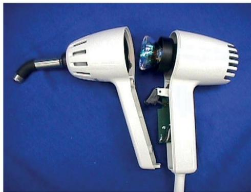
**Figure 13.** Internal components of a typical QTH curing light.
