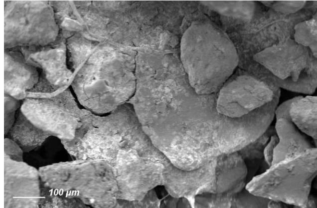
Figure 83 : SEM images of filter cake/surface mat above the media
