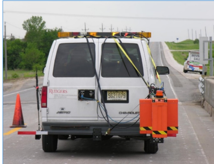
Figure 2.11: Example of a commercial Air-coupled GPR [6]
