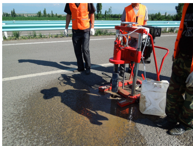
Figure 2.2: Coring equipment in [1]: the core cylinder is up to 200 mm in diameter and the complete setup can weigh up to 110 kg.
