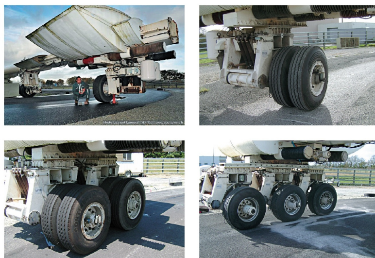
Figure B.8: Carousel loading arm configurations at the fatigue carousel at IFSTTAR
