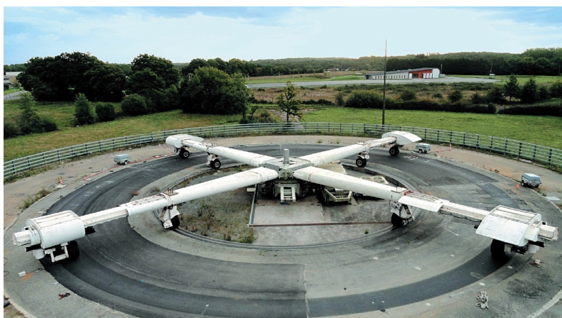
Figure B.7: Fatigue carousel at IFSTTAR, Nantes site [15, 16]
