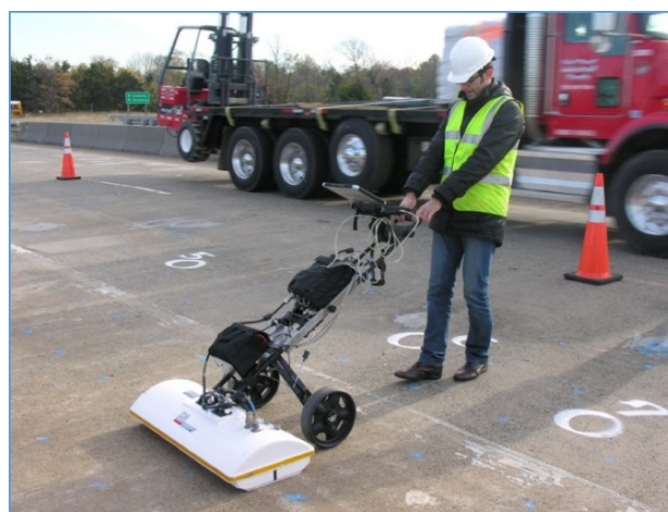
Figure 2.10: Example of ground coupled GPR [6]
