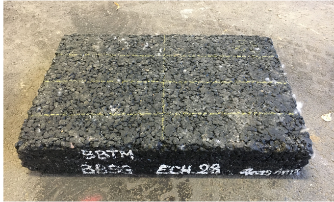
Figure B.2: A bituminous concrete test slab used during the experiments [13]
