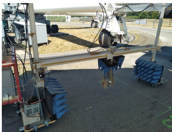
Figure 2.7: Data collection at the fatigue carousel at IFSTTAR using a pair of robot-controlled bistatic antennas
