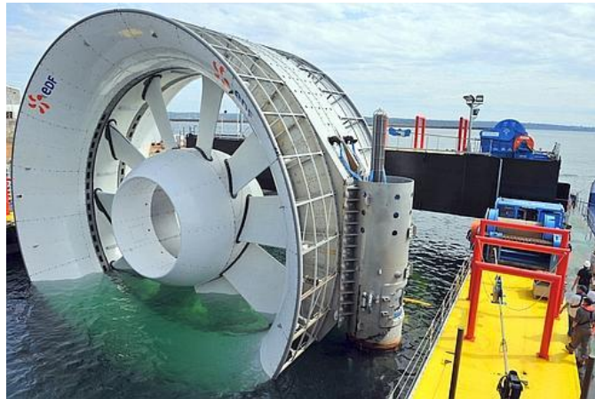
Figure I-3 : Hydrolienne OpenHydro 500kW
