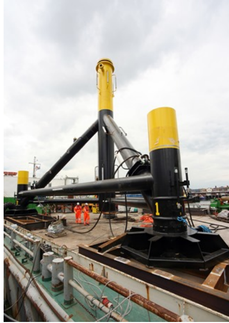
Figure 3.6 – Structure de support de type tripode d’EMEC FORESEA
