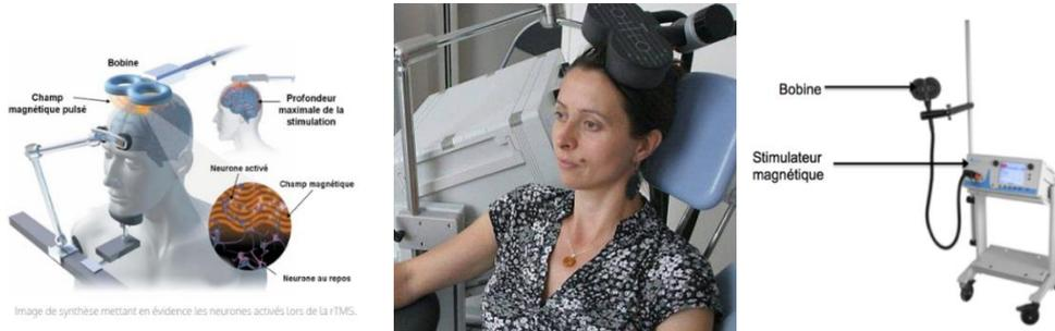
Figure 7 : Appareils de rTMS. <https://machine-neuroad.weebly.com/la-stimulation-magneacutetique-transcracircnienne.html>
