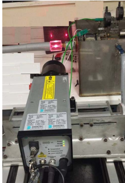
Figure IV- 1 Instantaneous velocity measurement through FlowExplorer laser Doppler anemometer
