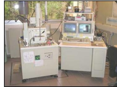
*Figure 29 MEB JEOL ltd 5800V
