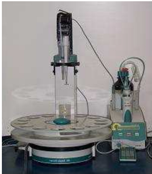
Figure B.9: The potentiometer titrator
