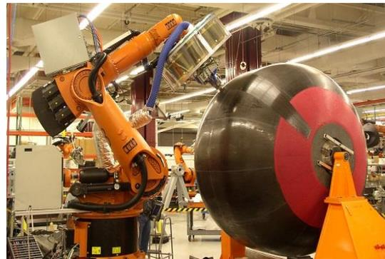
Figure 2.15 Surfaces complexes en composites
