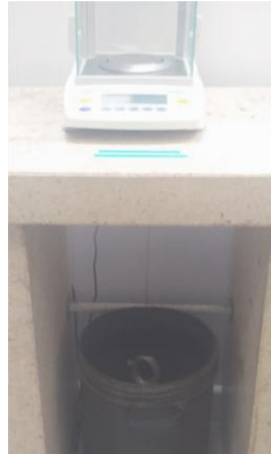
Figure 2.6. Weighing scale for immersed materials with a suspended rope sample.
