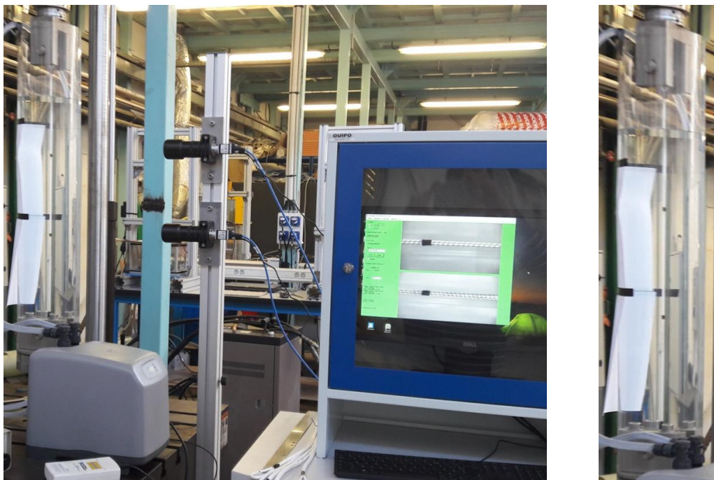
Figure 2.9. Testing device for dynamic tension-tension on immersed ropes: global view [left] and zoom on tube and end connexions [right]
