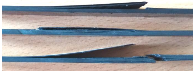
Figure 4.13. Sample failures after four point bending tests on aged 0/90° composites.
