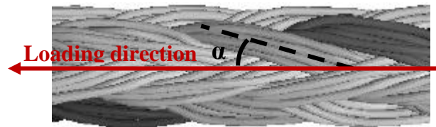
Figure 3.19: Representation of the average angle of filaments ( \alpha ) to the loading direction, defined to be equal to the braided angle.
