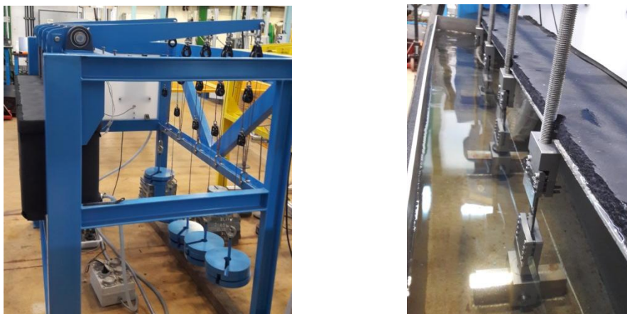
Figure 2.2 Testing device to study static tensile loading effects of water diffusion
