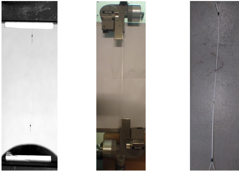
Figure 2.5. The different samples for quasi static testing on filament [left], yarn [middle] and rope [right]
