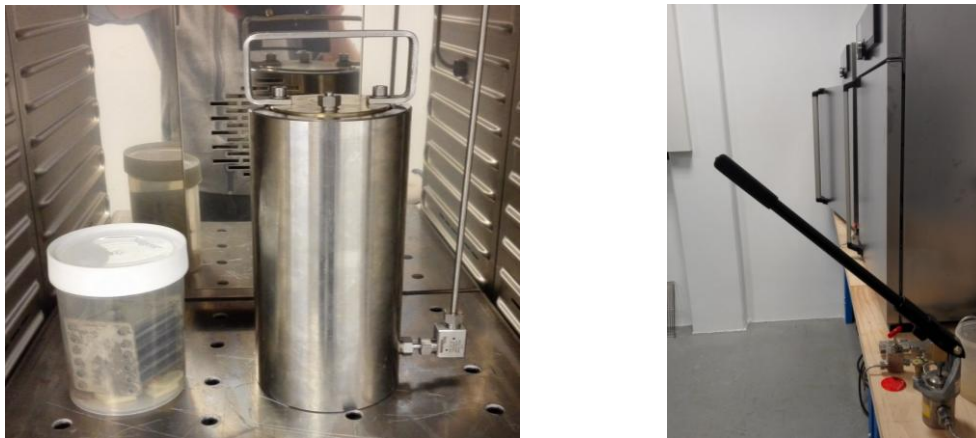
Figure 2.3. Pressure vessel in the oven [left] and the hand pump device to apply pressure [right]
