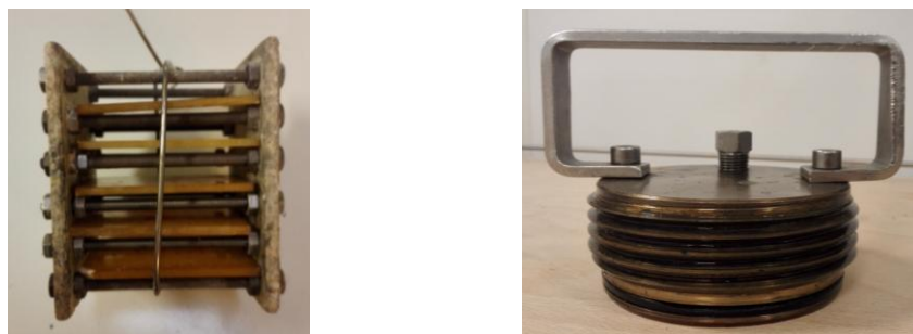
Figure 2.4. Specimens' rack used in the pressure chamber [left] and the specific lid employed [right]
