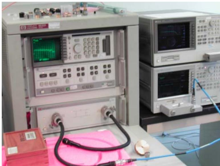
**Figure 10.** The experimental device consisting of a network (left) analyzer and an impedance analyzer (right).
