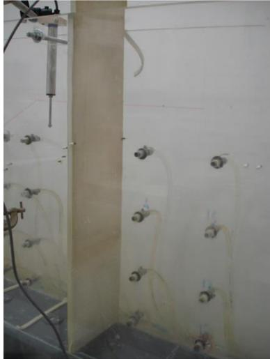
*Figure III.4 Fibre mess to separate dike soil and upstream water reservoir*
