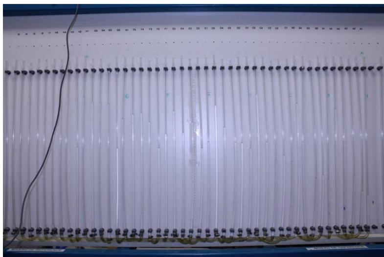
**Figure III.9 Measurement system: water head pipes**
