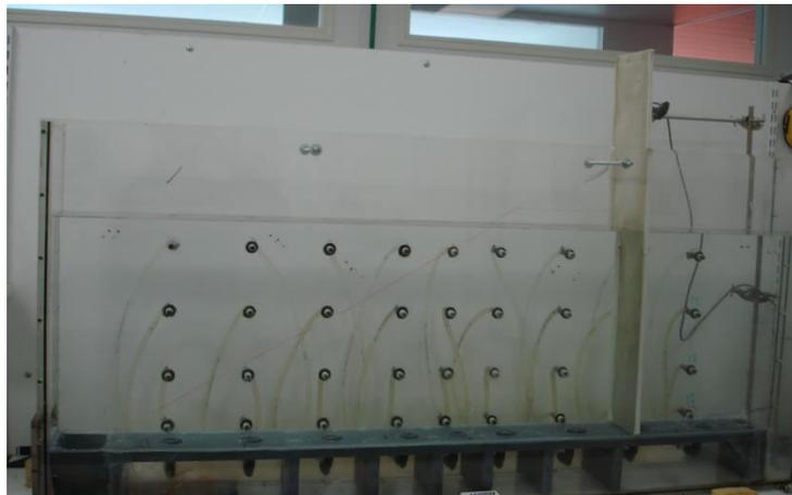
*Figure III.15 Saturation process of water pressure ports*
