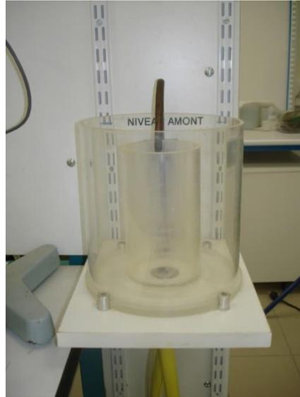
*Figure III.6 Upstream overflow outlet to maintain upstream water level*
