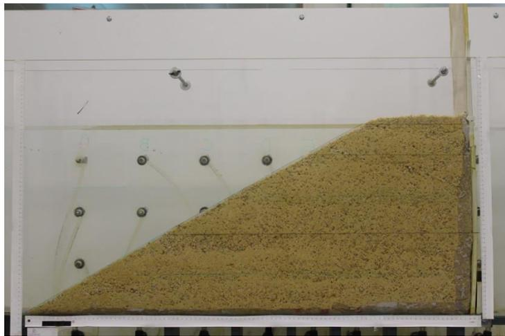
*Figure III.18 Saturation process of the specimen*
