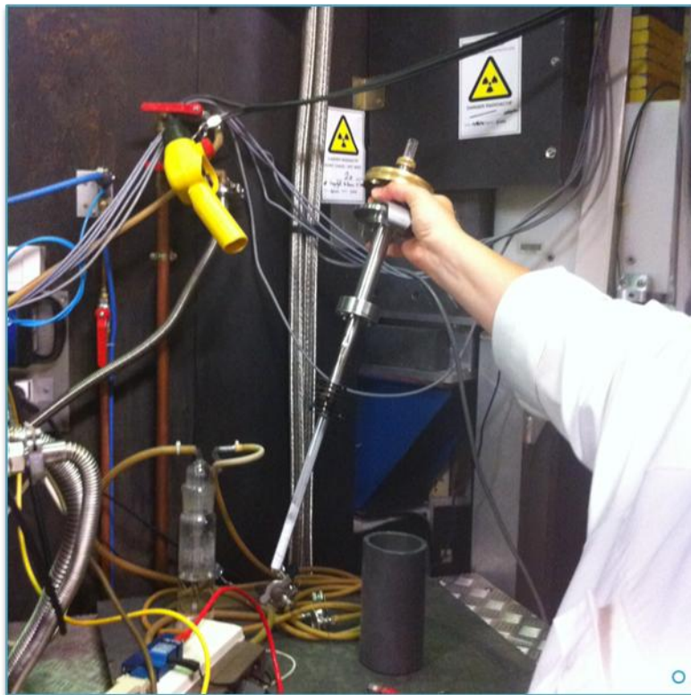
○ Quartz tube D2O bubbling ○○ Furnace (0-800°C) ○○○ Detector ○○○ Displex (4 K) ○○○ Vanadium
