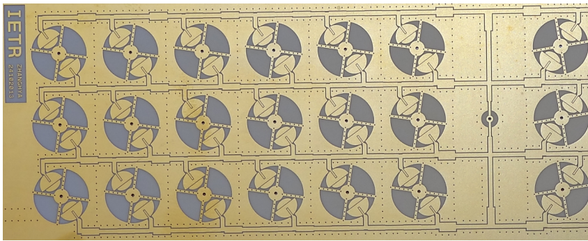
Figure 3.15: Photograph of 3x12 CPW-fed monopole antenna array (part) fabricated in 'PROTECNO GTID' PCB factory of Brest, FRANCE
