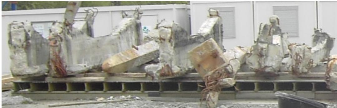
Figure 6.6 — Beams after 80 years of exposure.
